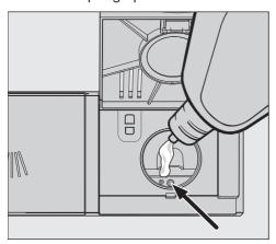
Fill with rinse aid until the filling level indicator (arrow) changes to a dark colour while the door is horizontally open.
